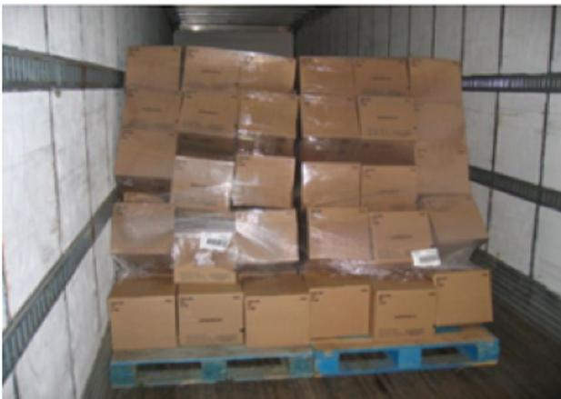
*An improperly loaded pallet can shift during transit, resulting in shipment damage and restacking costs. Source: [Lantech](#)*
