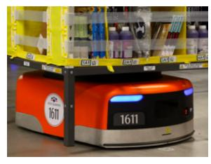
Amazon first introduced the concept with the deployment of a <u>fleet of robots</u> manufactured by Kiva (which Amazon later purchased) to automate the picking and packing processes at its warehouses. The Kiva robot, as described by <u>Business Insider</u>, "is a square-shaped machine that runs on wheels. They're about 16 inches tall and weigh almost 320 pounds. They can run at a steady 5 miles per hour and haul packages weighing up to 700 pounds."
