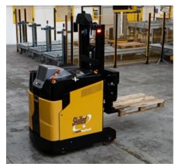
Driverless forklifts are also helping to transform warehouse and manufacturing floors. The concept of the driverless forklift is almost 60 years old, according to *Robotics Tomorrow*, when the idea was based on a forklift that followed an overhead wire. Today's driverless forklifts are "stepping into the future" and can approach a pallet, lift it, and then drive off to the next point, with no human assistance required.
