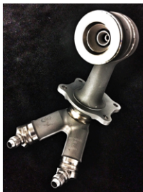
GE's 3-D printed fuel nozzle. Source: GE Reports
